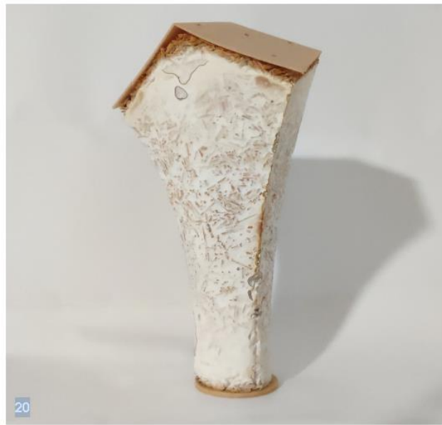
Figure 4. Building element from ganoderma lucidum mycelium cultivated in a hemp fiber substrate. One of the three types of building elements with different geometry produced in the context of a Diploma Thesis in the Department of Architectural Engineering.
