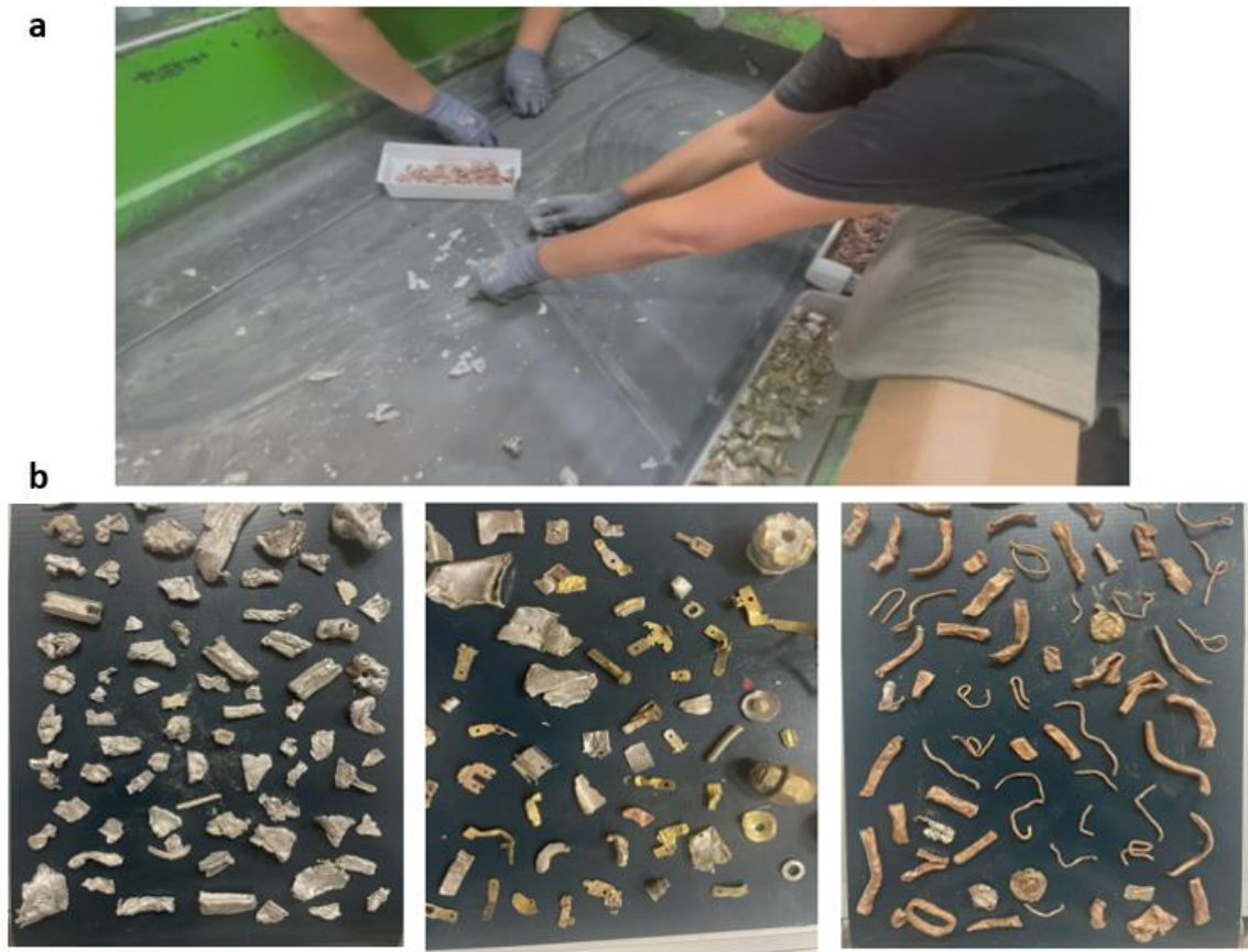
Figure 4. Manual sorting of ferro-neutral metals (a) and recycled samples (b).
