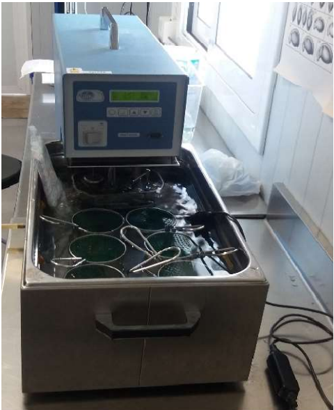
Figure 1. Experimental design used (Steel tank, baskets and digit cool thermostat) to measure the CTmax and cold tolerance of Calotriton arnoldi .
