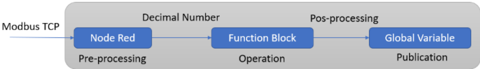
Figure 5. Internal data process flow used in the PLC.
