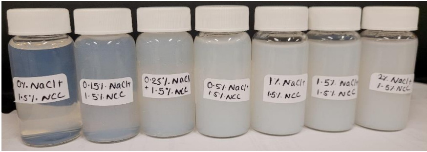
Figure 22. Appearance of 1.5 wt% NCC dispersion samples with the addition of salt (NaCl).
