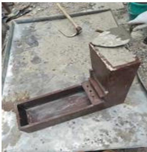
Figure 3(c) L-Box Test
