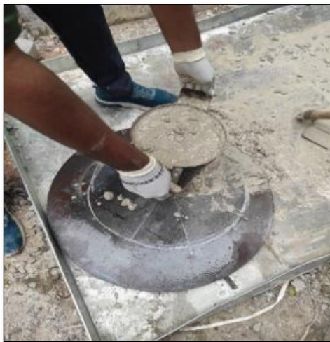
Figure 3(a) Slump flow
