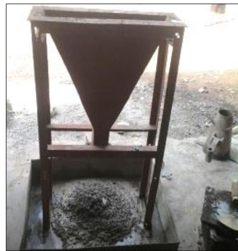
Figure 3(b) V-Funnel Test
