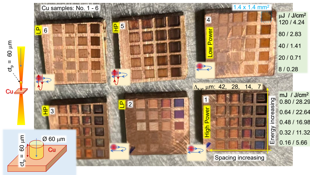
Figure 2. Typical 1 \times 1 \text{ cm}^2 coupon-samples (Cu) used for determination ablation rates. Samples are not polished. High and low power ranges were used to explore the different surface roughness and material removal rates of ablated surfaces, see, pulse energy E_p and fluence F_p [ \text{J}/\text{cm}^2 ]. F-theta lens had focal diameter on the sample 2r = 60 \text{ μm} , depth of focus \text{DoF} = 2.7 \text{ mm} , field of scan 50 \times 50 \text{ mm}^2 , and axial pulse extent of ct_p = 60 \text{ μm} for pulse duration of t_p = 200 \text{ fs} . The melting temperature of Cu is 1085^\circ\text{C} , evaporation/boiling 2595^\circ\text{C} . For samples No. 1, 2 the focal spot was placed 6 mm deeper along beam propagation from the top surface of the sample. Hatching passes in x-/y-directions are schematically shown; the total number of passes was always 10.
