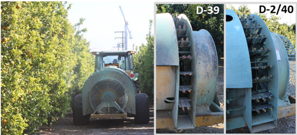
Figure 1. In-progress spray application inside orchard during the study and views of nozzle banks on the two sprayers used.
