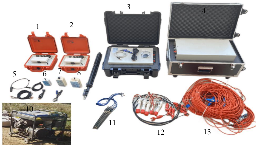
Figure 2. Materials used for the SSIP survey. (1) GS2IP-FW10 Full Waveform SSIP Receiver, (2) GS2IP-FW13 Full-waveform SSIP current acquisition station, (3) SSIP transmitter, (4) GSTP series programmable DC power supply, (5) Receiver power cord, (6) Receiver wireless control box, (7) Current converter, (8) Receiver relay station, (9) Tripod, (10) Power generator, (11) Brass electrodes for current injection, (12) Non-polarizable Pb-PbCl 2 electrodes, and (13) SSIP receiving cable.
