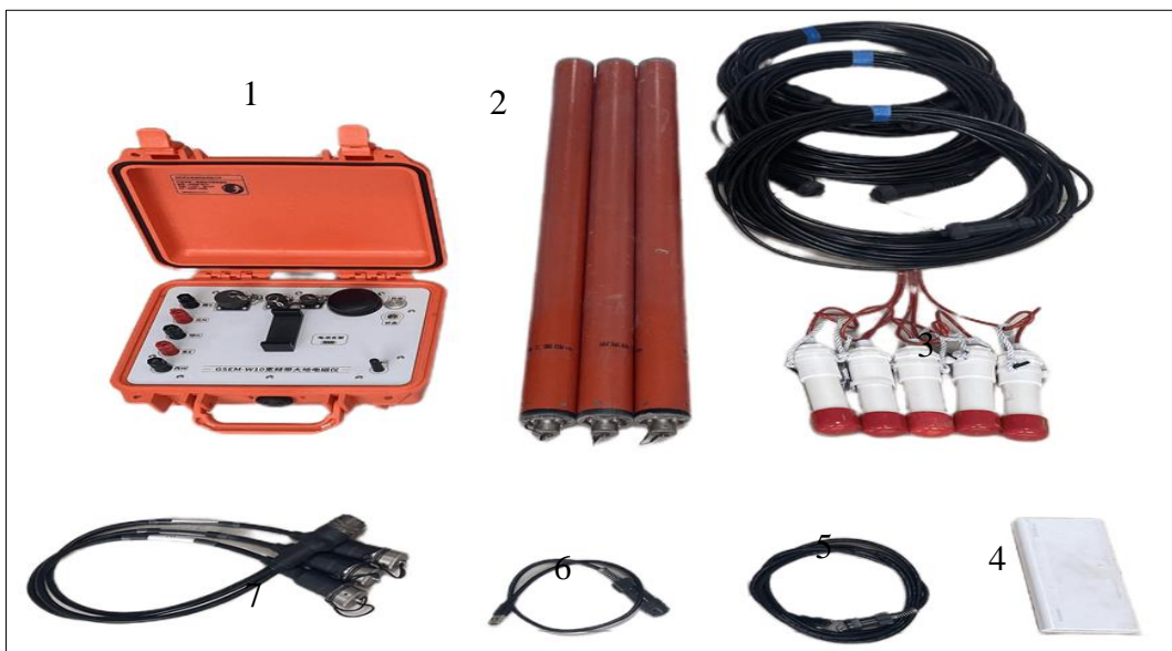
Figure 3. Materials used for Audio magnetotellurics survey. (1) GSEM-W10 AMT acquisition units; (2) Induction Coil Magnetometers (ICM); (3) Non-polarizable Electrodes; (4) Portable power bank; (6 and 7) Connecting field cables.
