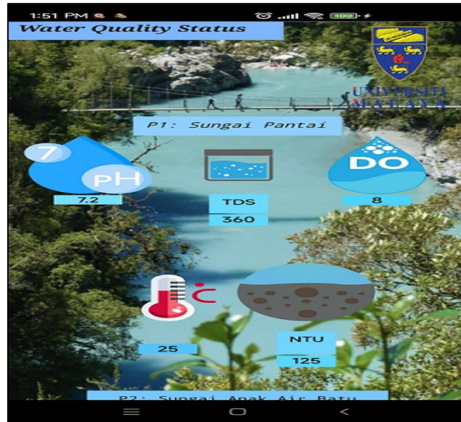
Figure 7. Water Quality Monitoring Dashboard in Android View.
