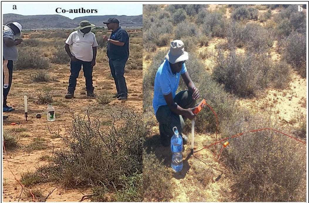
Figure 5. a and b: Field procedures of the ground magneto-telluric surveys during the investigations.
