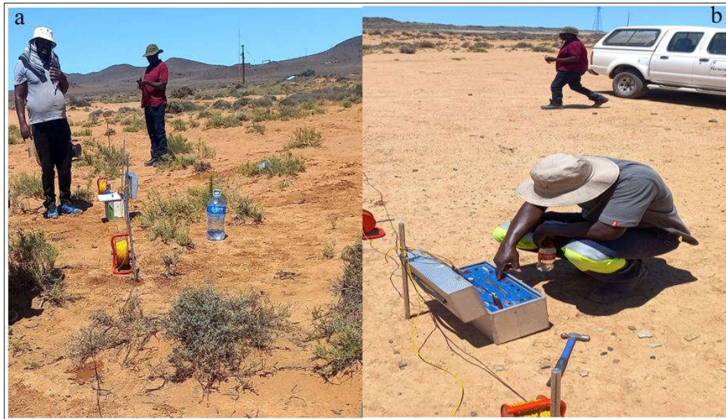
Figure 3. a, b, and c: Field setup of the electrical resistivity survey during the field investigations.
