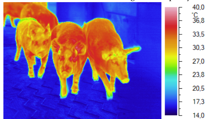
Figure 4. Monitoring the skin temperatures of pigs as they arrive at the slaughterhouse.
