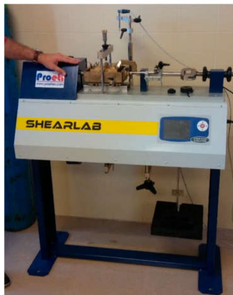
Figure 4. Direct shear device available at the geotechnical laboratory.
