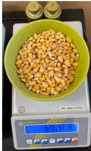
Figure 3. Electronic balance of 0.01 g accuracy used in the determination of moisture content.
