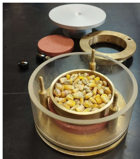
Figure 6. Oedometric cell used with the maize sample.
