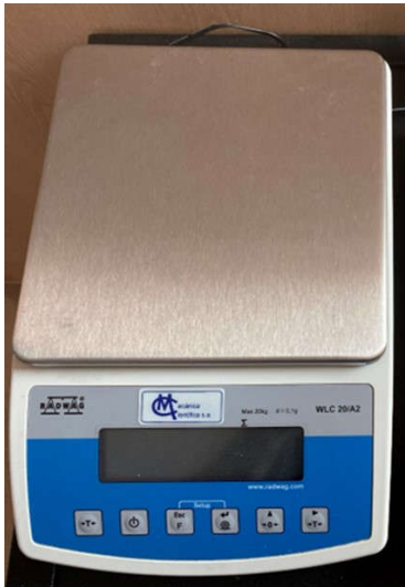
Figure 7. Electronic balance of 0.1 g accuracy used in oedometric assays.
