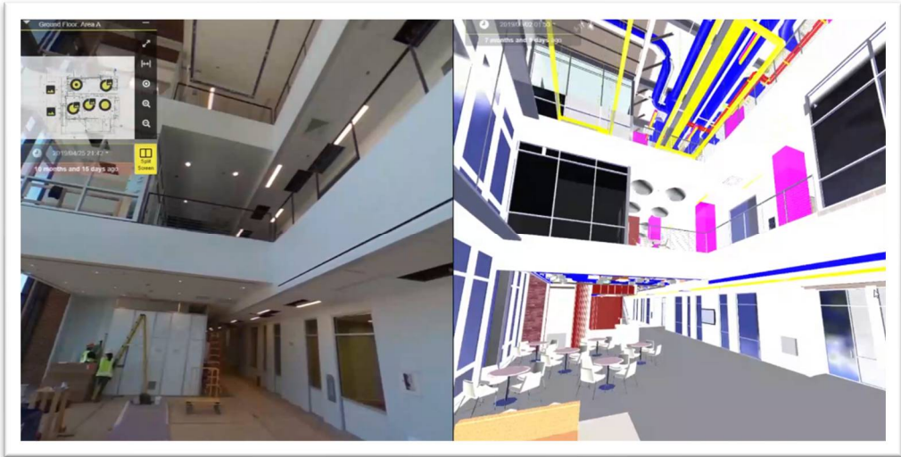
Figure 8. Construction Documentation Using HOLOBUILDER Platform. The left image is captured using 360° cameras. The right side indicates the same scene in the BIM model.
