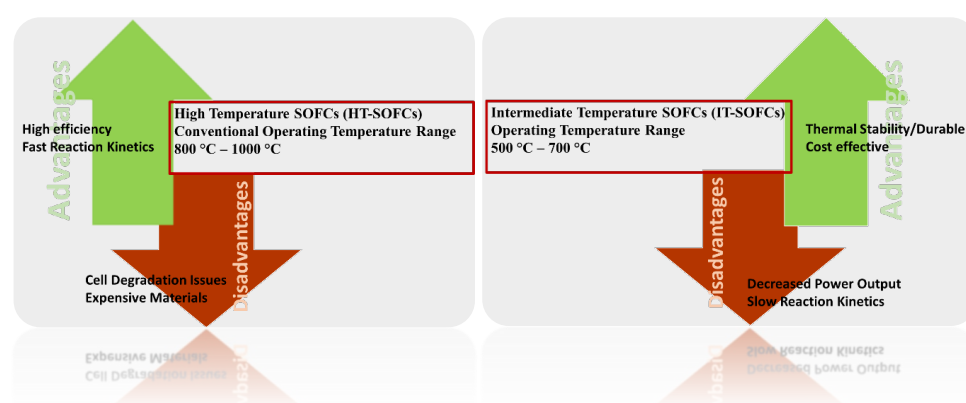
Figure 3. Comparison between Intermediate and High temperature SOFC.
