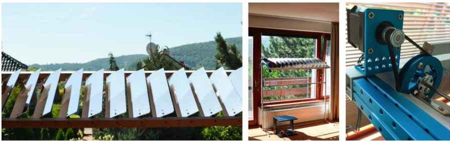
Figure 12. The combination of a light shelf with a set of mirrors [9].
