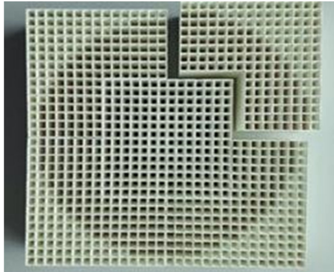
Figure 1. Whittaker et al. 3D-printed perorated dielectric transmitarray (TA) with total dimensions of 180 \times 180 \times 32 mm.
