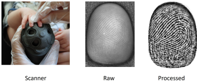
Figure 2. Synolo® Neo scanner and fingerprint of two months infant.
