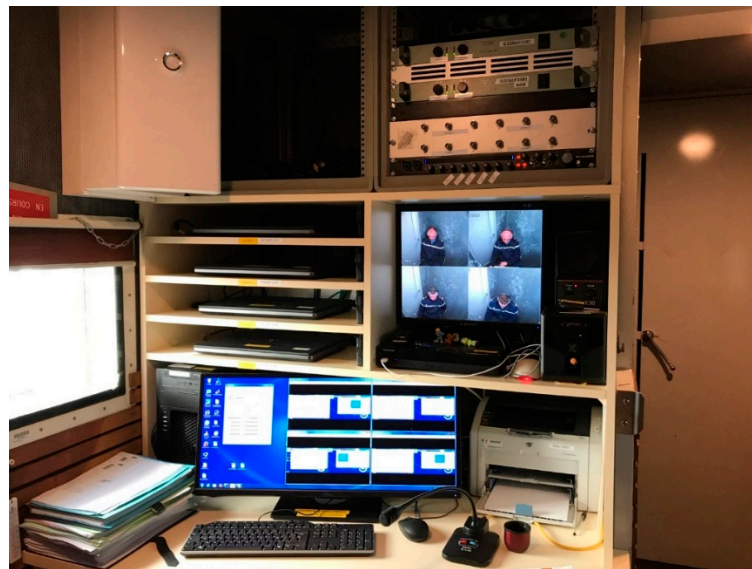
Figure 3. Interior view of the Mobile Hearing Laboratory. In the center right of the setup, a video screen displays images of participants situated in the four booths. Positioned in the center left are four portable "followers" computers equipped with fold-down screens, to which the screens, keyboards, and mice of each booth are connected. Beneath these computers, there is the "leader" computer, positioned at the bottom center, with its screen visible. Additionally, the screens corresponding to the "follower" computers are also visible.
