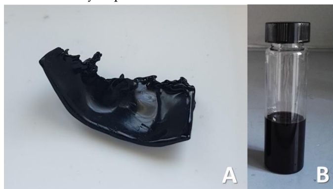
Figure 1. Piece of PA product as isolated from the reaction medium (a) and absolute sulfuric acid containing the dehydrated PVOH oligomers (b).
