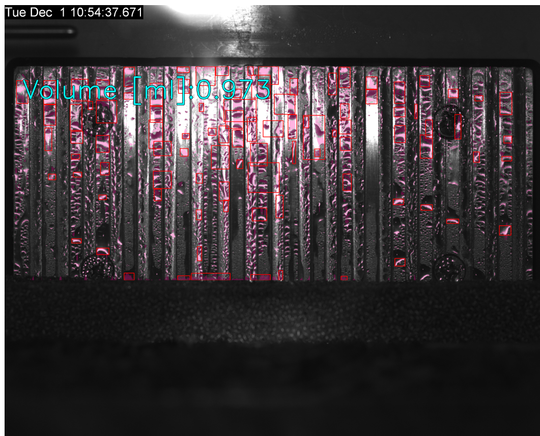
Figure 9. Example of the volume quantification on grooves
