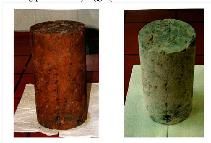
Figure 3. Image of whole diameter core from the Vranovice carbonate formation for well ZA4A, depth 1781 – 1781.3 m. The left image displays a core sample before and right image after cleaning and drying.
