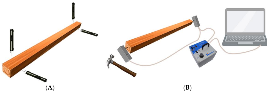
Figure 3. Wood hardness test scheme for wood samples (A) and wood propagation speed measurement by ARBOTOM 3D (B).
