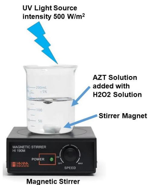
Figure 2. An aqueous solution containing AZT and H 2 O 2 on a magnetic stirrer cum hot plate, irradiated with UV light having 500 W/m 2 intensity, input voltage 230 V, and 50/60 HZ.
