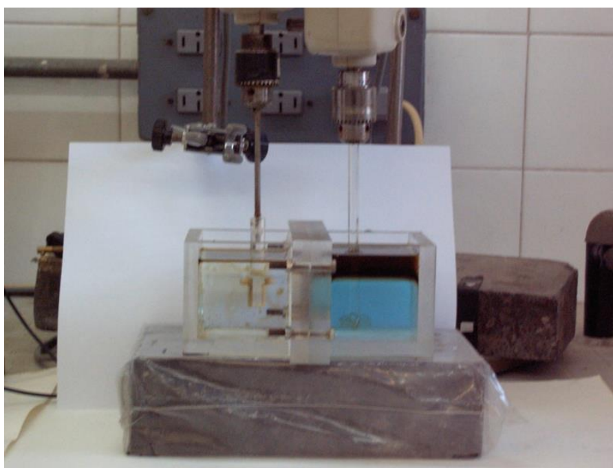
Figure 3. Non-dispersive extraction with strip dispersion. Phases at the end of the operation. It can be observed the transport of the metal (blue color) from the feed to the strip phase.
