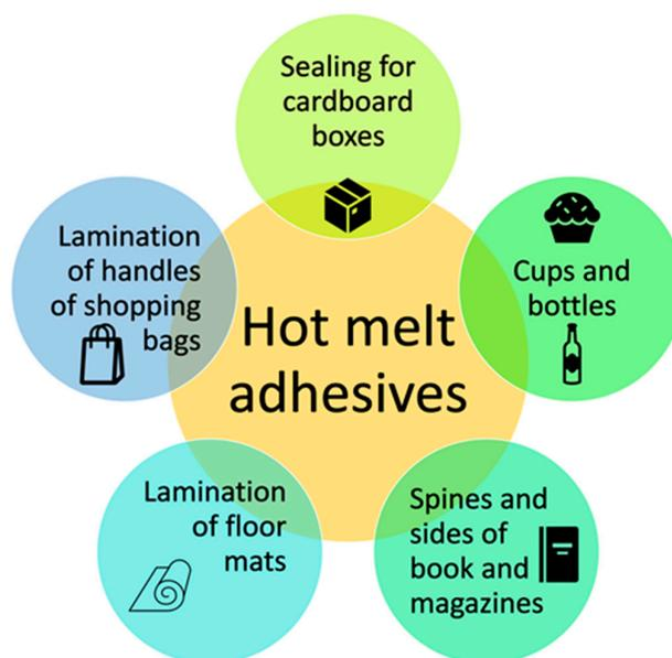
**Figure 10.** Common applications of hot melt adhesive.
