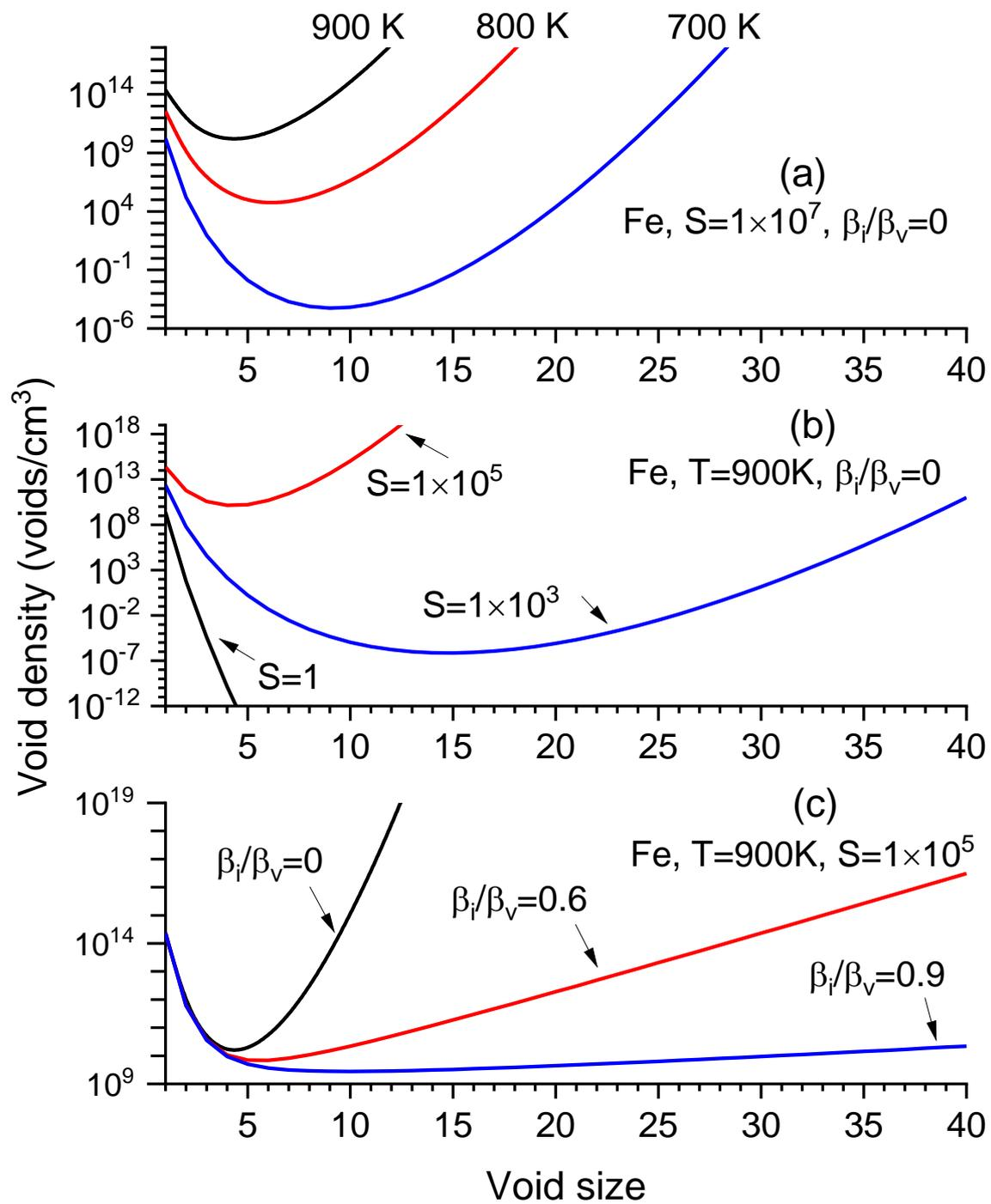
**Figure 1.** Void density as a function of void size (number of vacancies contained in a void) under various conditions in  $\alpha$ -iron: (a) different temperatures, (b) different  $S$  values, and (c) different  $\beta_i/\beta_v$  ratios.
