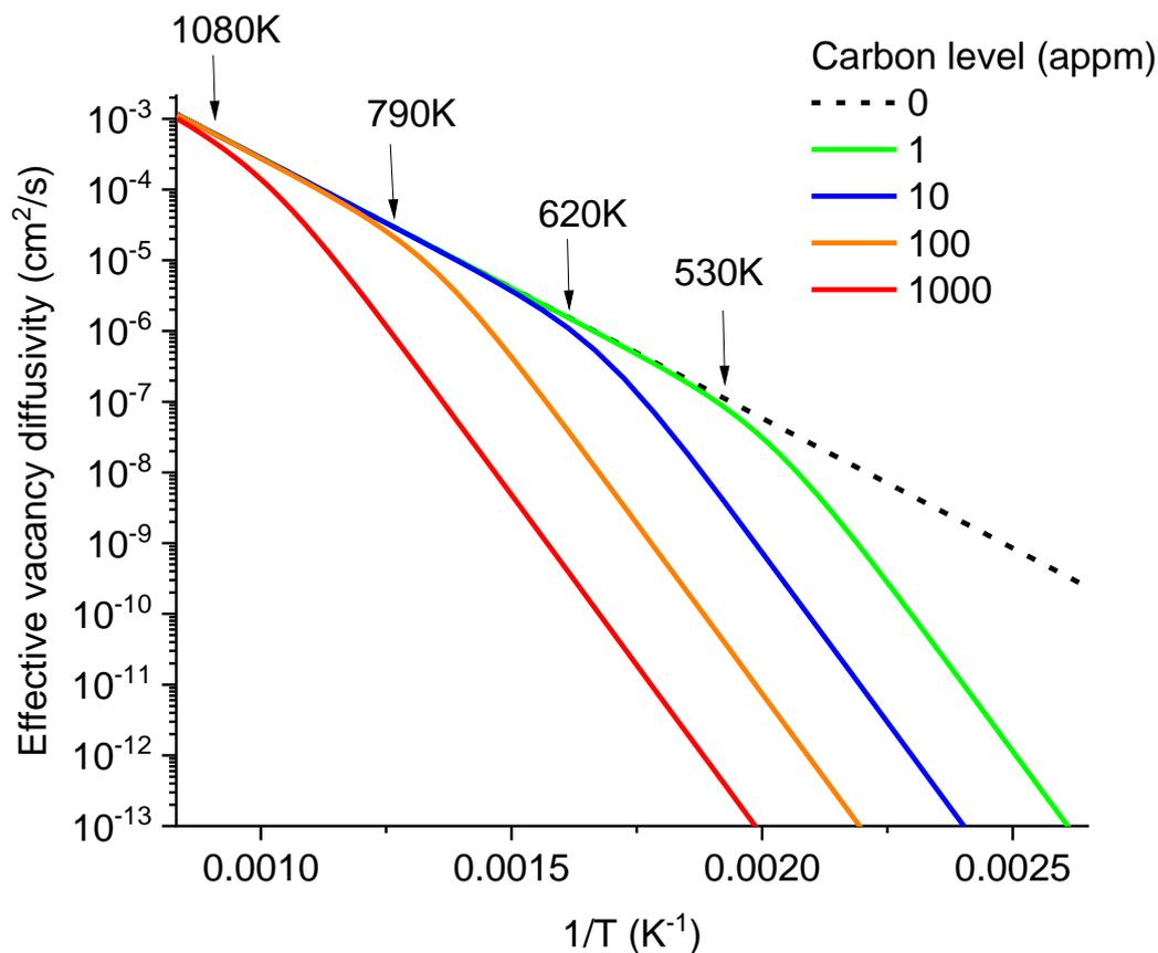
**Figure 4.** Effective vacancy diffusivity as a function of temperatures and C concentrations in  $\alpha$ -iron.
