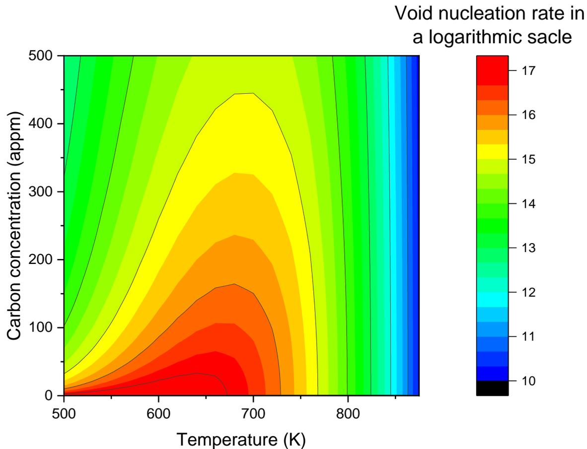
**Figure 5.** The map of void nucleation rates as a function of C concentrations and temperatures in  $\alpha$ -iron.
