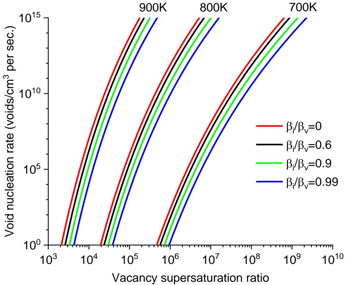
**Figure 2.** Void nucleation rates as a function of  $S$  at different temperatures (700, 800K, 900K) and  $\beta_i/\beta_v$  ratios (0, 0.6, 0.9, and 0.99).
