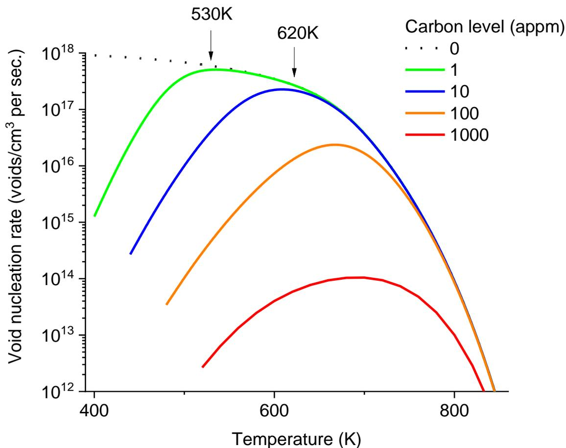
**Figure 6.** The plot of void nucleation rates as a function of temperature for C concentrations ranging from 0 to 1000 appm in  $\alpha$ -iron.
