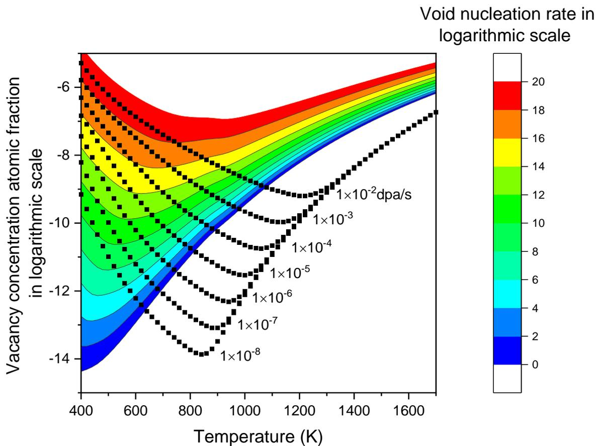
**Figure 3.** Vacancy concentration (atomic fraction, on a logarithmic scale) at different temperatures for various steady-state void nucleation rates (color contour), and under different dpa rates (square lines) in  $\alpha$ -iron. The point of intersection between a square line and a colored contour line gives the nucleation rate at a specific temperature and dpa rate.
