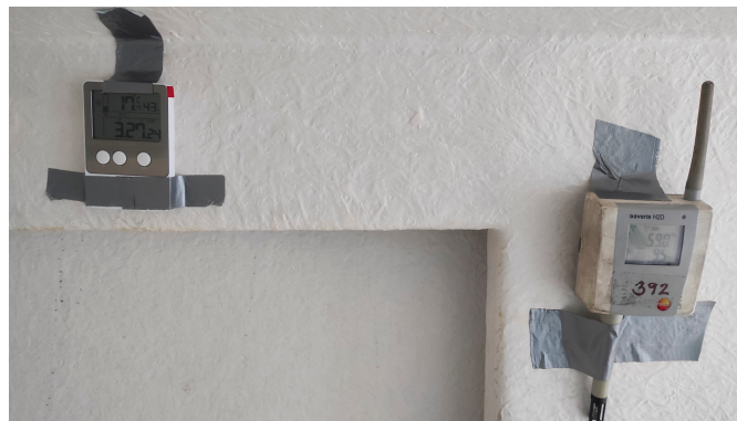
Figure 7. The control measuring equipment Hadex and Testo H2D.
