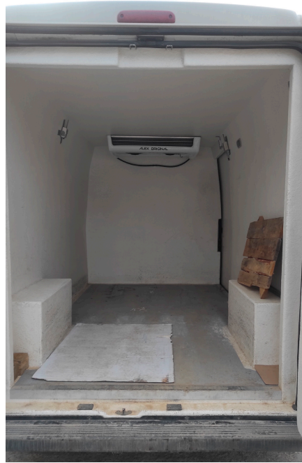
Figure 9 Adjusting the ALEX Original TRE24 vehicle-mounted refrigeration unit.
