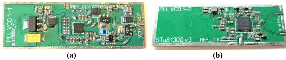
Figure 14. Photograph of manufactured prototypes (a) PLL1 and (b) PLL2.
