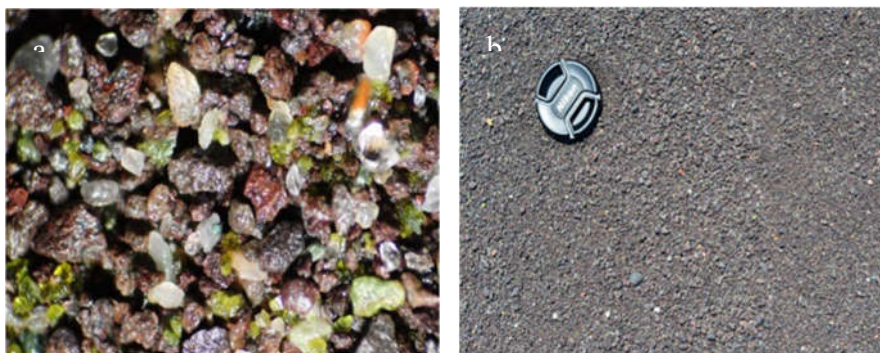
Figure 3. Stamp Sands in situ under natural sunlight: a) wet redeposited stamp sand beach deposits close-up (12.5 cm wide field), showing colored crushed gangue mineral grains and b) from a distance,
