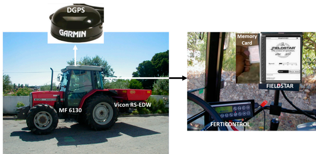
Figure 4. Previous solution to VRT (Variable Rate Technology) control of “Vicon RS-EDW” spreader with the “Massey-Ferguson 6130” tractor: details of GNSS antenna “Garmin 16”, and “Ferticontrol” and “Fieldstar” controllers (this with the memory card type “PCMCIA”).
