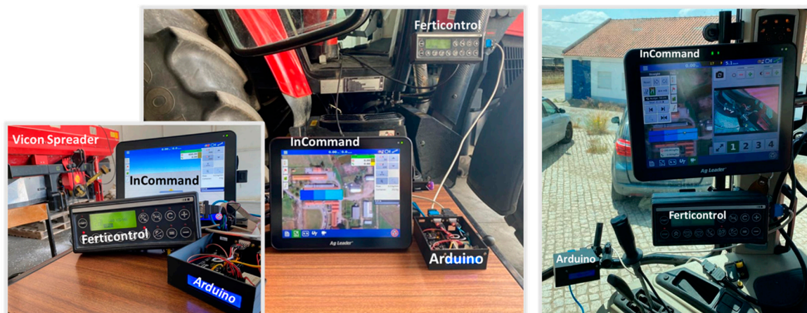
Figure 11. Proposed solution (“InCommand” – “Arduino” – Ferticontrol”) installed on the tractor.
