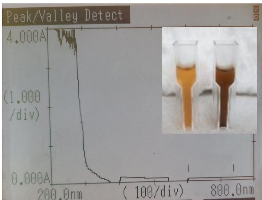
**Fig.S1.** UV-Vis spectrometry analysis of synthesized CCIO NCs
