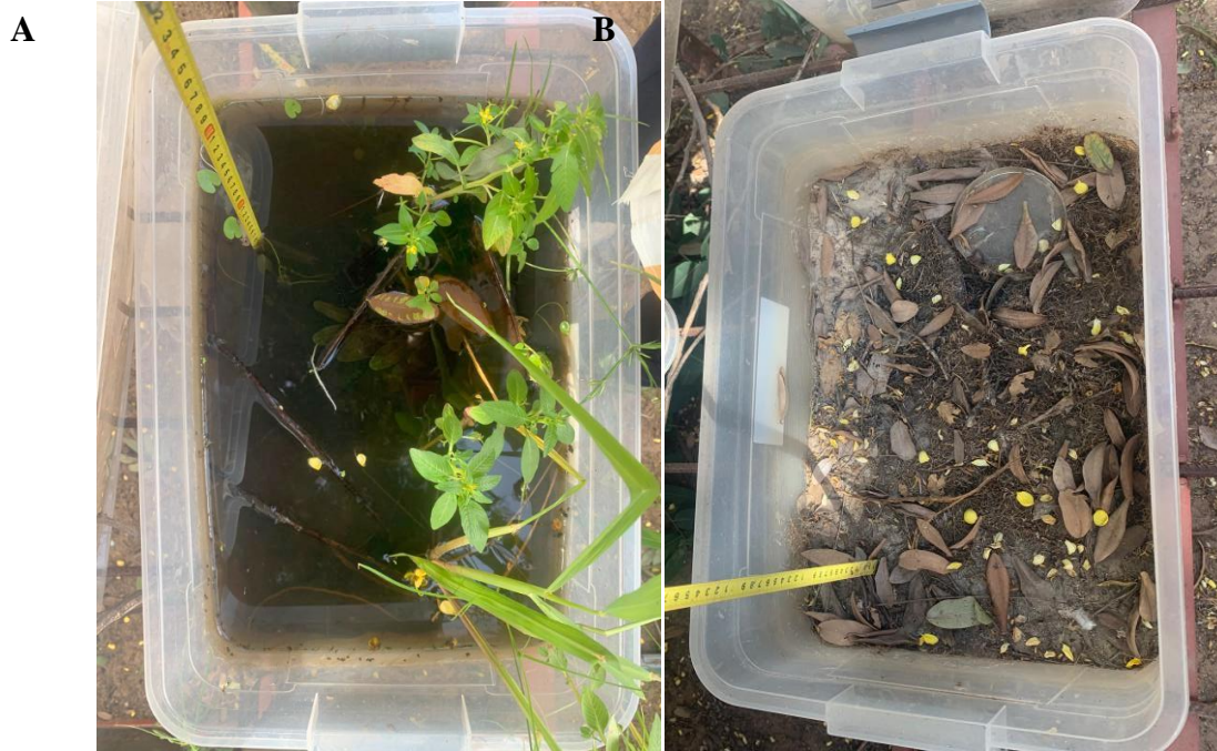
Figure 4. Tanks used to reproduce drought in semi-natural conditions. A) tank filled with water; B) tank dried out after to months.
