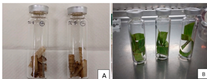
Figure 1. Thin strips of substrates were placed in 20 ml headspace glass vials prior to E-nose sampling. (A) Healthy and Tropical Race 4 infected banana pseudo stems, (B) Healthy and infected mango leaf samples.
