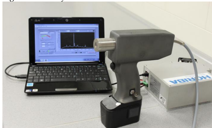
Figure 4. Portable Raman system. This figure shows the composition of the portable Raman system. Note: Handheld Raman device (center), miniaturized spectrometer (right), and netbook (left).
