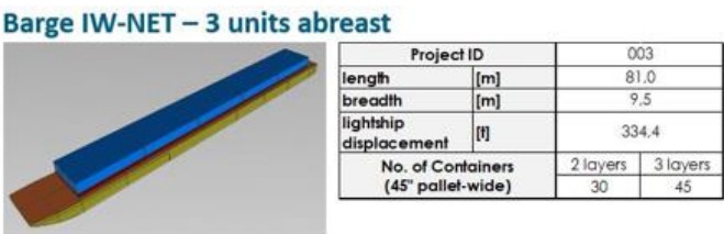
Figure 2. CAD model and details about "IW-NET - 3 units abreast" barge design.
