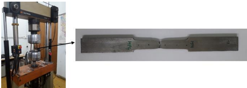
Figure 4. Tensile test equipment and coupon test specimen after fracture.
