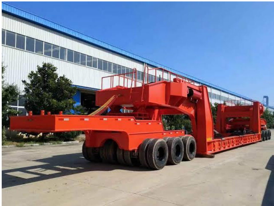
Figure 8. Module Loading (towed hydraulic platform trailers and self-propelled hydraulic platform trailers).
