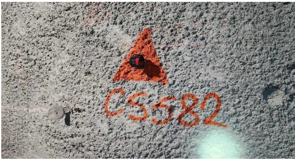
Figure 2. The mark of the central point of the network.
