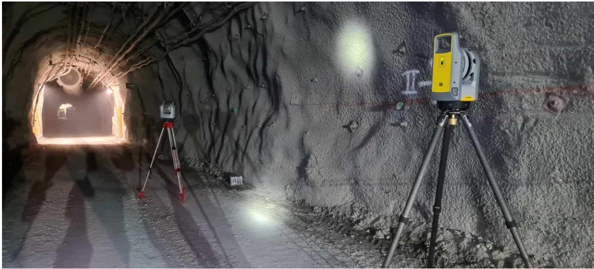
Figure 3. TLS measurement of cross section in the underground mining tunnel.
