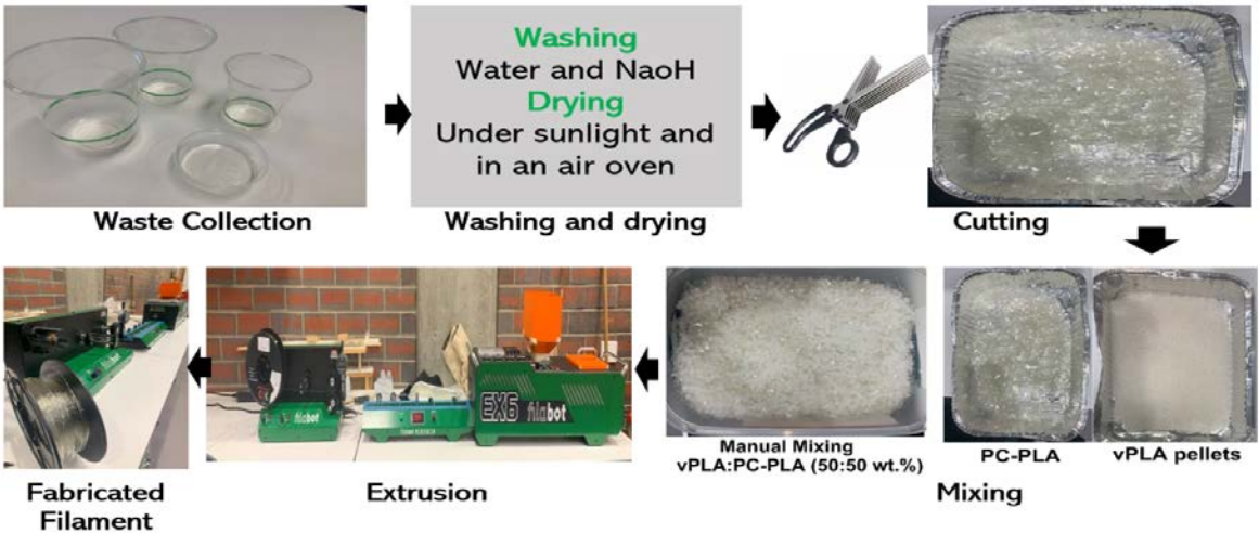
Figure 4. Illustration of the process followed for blend filament production.
