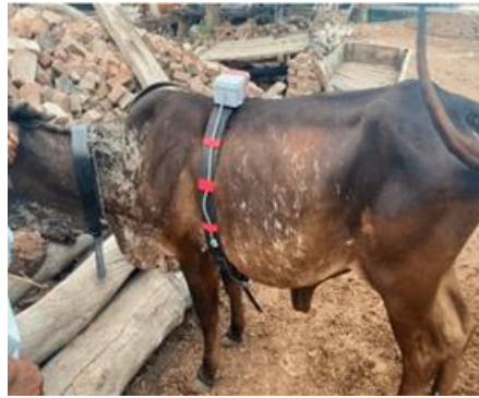
Figure 6. Intelligent Animal Monitoring System by using stethoscope.
