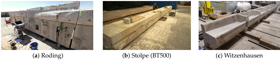
Figure 2. Bridge girders tested under laboratory conditions: (a) in-situ cast, post-tensioned element of the web of a hollow-box bridge near Roding, (b) prefabricated post-tensioned element (BT500) from a bridge near Stolpe and (c) prefabricated, pre-stressed element with single wires from a bridge near Witzenhausen.
