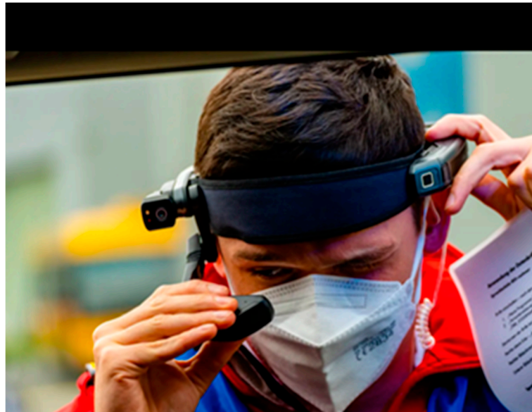
Figure 1. virtual Burn Assessment Teams (vBAT) by use of IRIS (Instant Remote Interactive Support“ ® Stryker, USA. The investigator has a camera attached to his head and a mini-monitor in his hand where evaluations from distant colleges can be seen.
