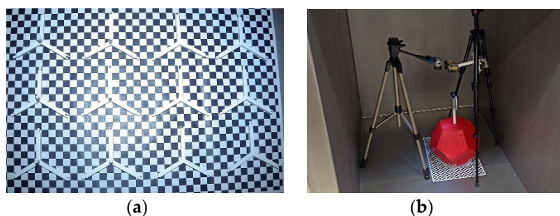
Figure 5. 3D printed parts (a) and the whole dodecahedron formed structure (b) inside the low air pressure chamber.
