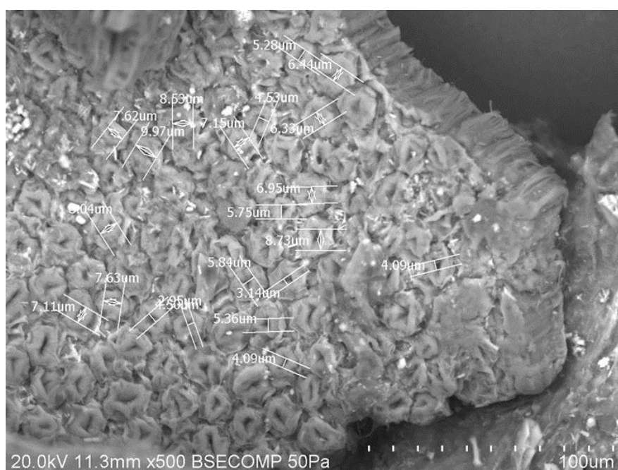
Fig. S17. SEM images and pore size measurements for the HTC 120 sample: A) Open pores; B) Pores in the process of forming.
