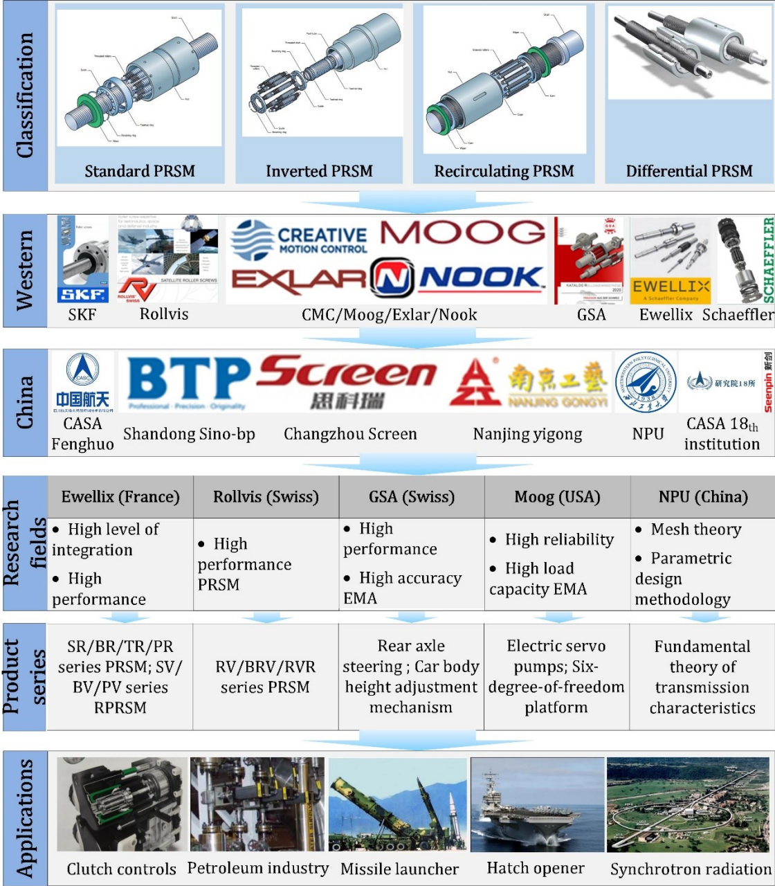
Figure 1. Classification, industrial status and applications of planetary roller screw mechanism. (Images from Bing).
