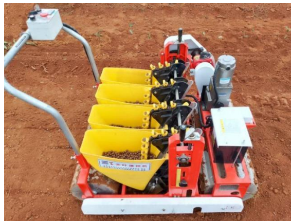
Figure 8. Tea seed planter and test site.
