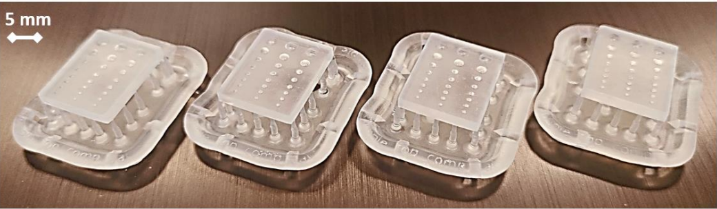
Figure 14. Picture of the four samples with variable compensation. Each sample has three patterns of micro-pores with varying diameters, from 2mm down to 500µm.
