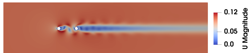
Figure 5. Two cylinders in tandem with an instantaneous depiction of the magnitude of the primal velocity.
