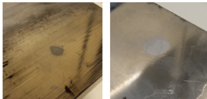
Figure 4. Sample of aluminum post-manual polishing. The image highlights the differences in surface finishing, with particular attention to the unpolished areas intentionally restored to detect typical material defects. This images was used for the network training, demonstrating the necessary contrast for accurate defect identification.
